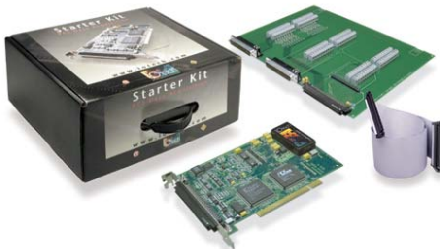
The DaqBoard/2000 Starter Kit includes DaqBoard/2000, DaqView2000 software, DBK202, and CA-195 cable
